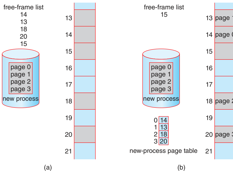
Figure 9.11 Free frames (a) before allocation and (b) after allocation.
