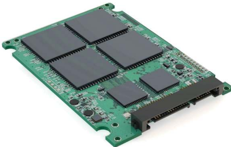
Figure 11.3 A 3.5-inch SSD circuit board.
