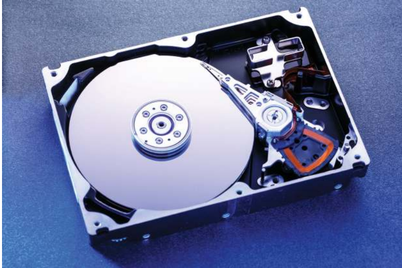
Figure 11.2 A 3.5-inch HDD with cover removed.
